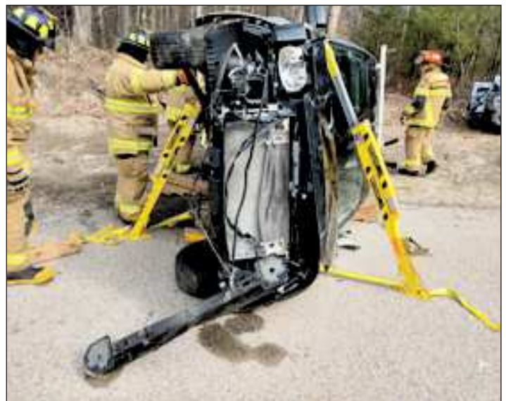
Locating Batteries to De-energize the Vehicle
